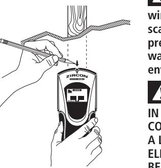
*Note: The tool may detect other objects behind the wall such as pipes and conduit. See Section 2: Operating Tips for ways to confirm that you found a stud.*
