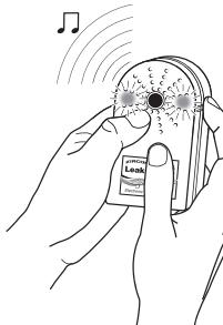
In the event of low battery, water detector will chirp (short beep every 5 seconds). Please replace with brand new 9V battery immediately.
