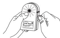
A loud, repetitive series of beeps will sound and the LEDs will flash red. Dry the contacts to stop the alarm.
