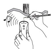
To avoid surprises, remember that studs or joists are normally spaced 400 mm or 600 mm apart and are 35 mm to 45 mm in width. Anything closer together or a different width may not be a stud, joist, or firebreak.
